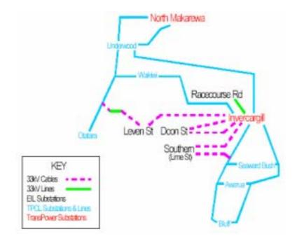
Figure A2.7 Electricity Invercargill Distribution Network
