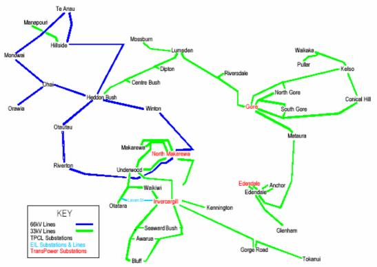
Figure A2.5 The Power Company Distribution System
