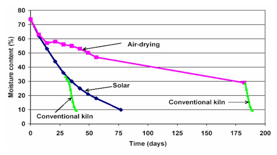
Drying times for air, conventional and solar drying and in combination for 30mm thick green boards of blackbutt. (Haque 2002)
