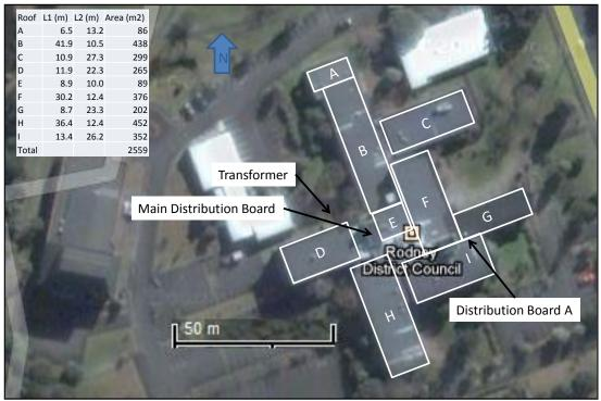
**Figure 8:** Approximate roof areas of Pacific Building only (does not show Tasman Building, white roof areas are temporary premises no longer existing) and location of some electricity supply infrastructure
