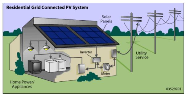
Figure 2: Residential Grid Connected PV system
