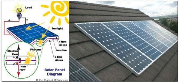
Figure 1: Solar panel diagram and installed on residential roof
