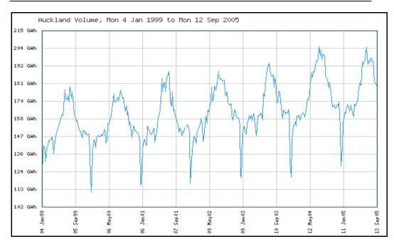
Figure 8 – Seven Year Electricity Consumption Profile
