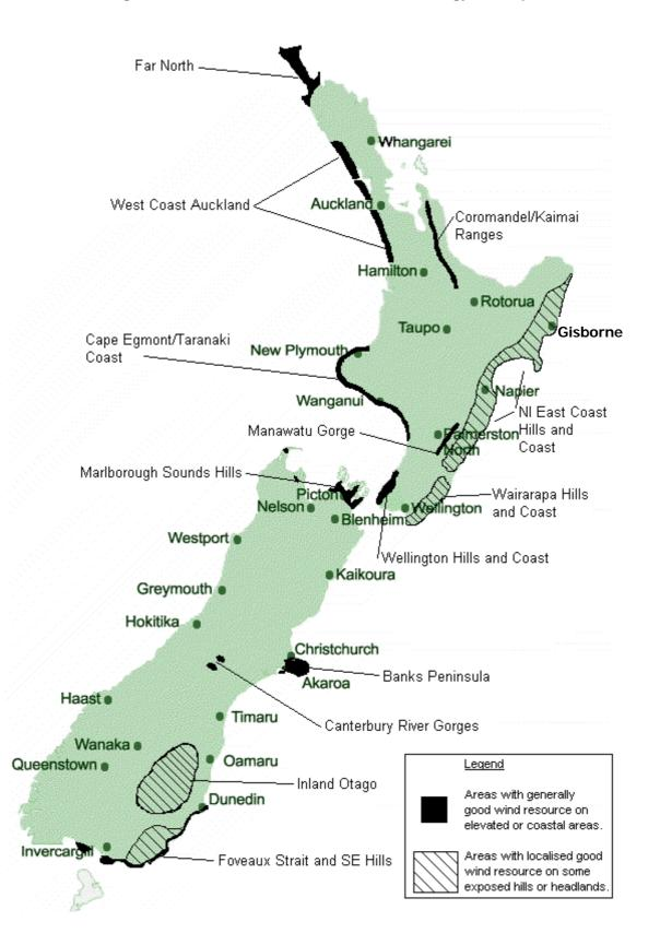
Figure W1: Location Most Suitable For Wind Energy Development
