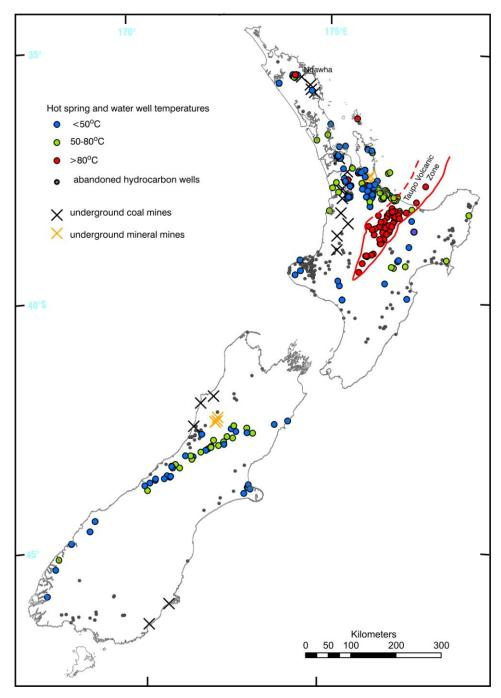
**Figure 2.2.** Location map of some geothermal sources including hot spring systems and their maximum surface discharge temperatures, abandoned onshore hydrocarbon wells and abandoned flooded underground coal and mineral mines (Reyes, 2007).
