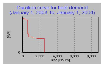
Figure 4.6. Heat duration curve for a primary school with heat covering space heating and a heated swimming pool.
