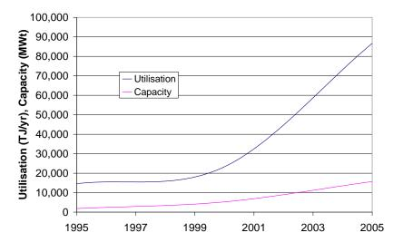
Figure 4.4. Illustration of the accelerated worldwide uptake of geothermal heat pumps over the last decade (data from Lund et al 2005).
