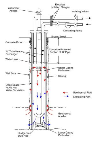
Figure 3.3: Typical down-hole heat exchanger with promoter tube casing (Thain et al 2006)
