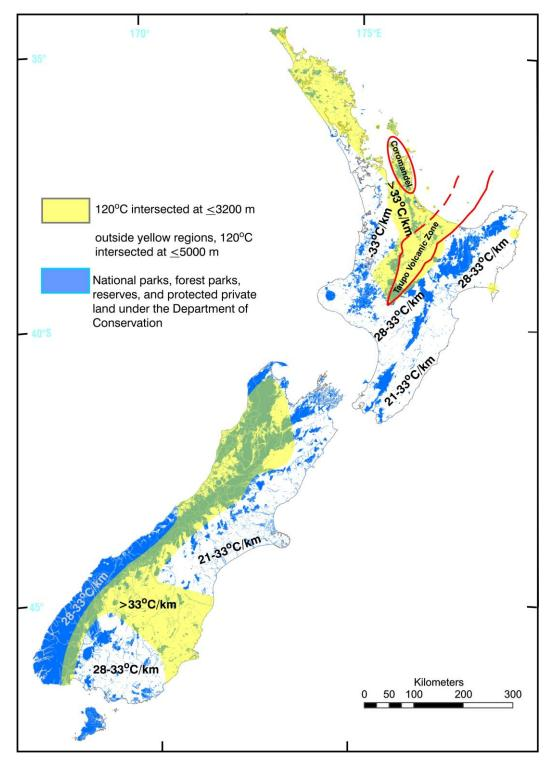
Figure 2.3. Areas used in calculating the minimum potential heat energy in the rock using shallow and deep-seated conductive heat (Reyes 2007).
