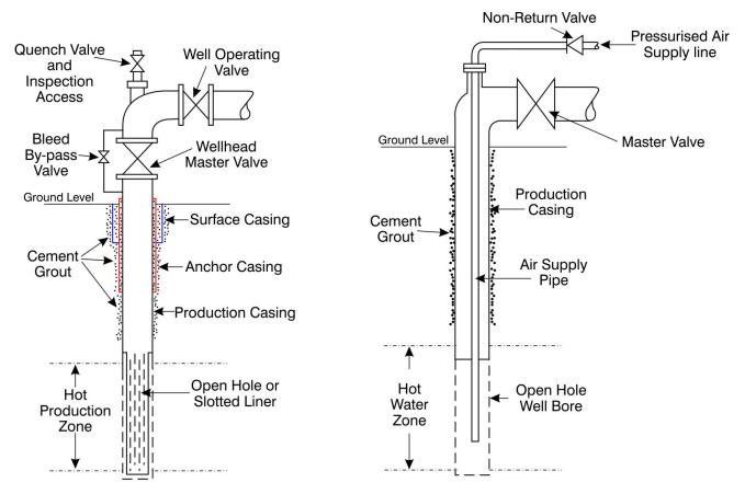
Figure 3.1. Typical wellhead and casing arrangements for pressurised and non-pressurised wells (Thain et al 2006)
