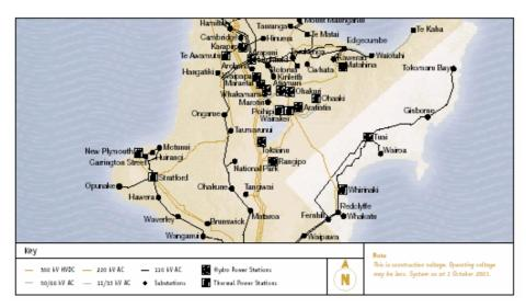
Figure 2 Schematic of the Transmission Grid for the Tairawhiti Region<sup>13</sup>
