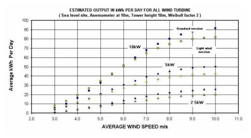
Figure 30 Estimated output in KWh per day for all wind turbines
