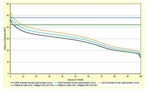
Gisborne Load Limits and Forecast Load Duration Curves<sup>15</sup> Figure 4
