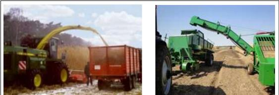
Miscanthus giganteus harvested using a modified forage harvester mounted on a combine, and rhizome lifting and splitting plant (US).
