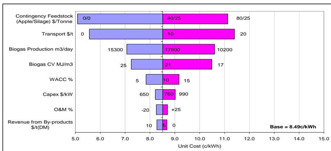
Figure 34 Cost of Biogas Production From Clustered Food Processor Group (80,000 tonnes p.a.).
