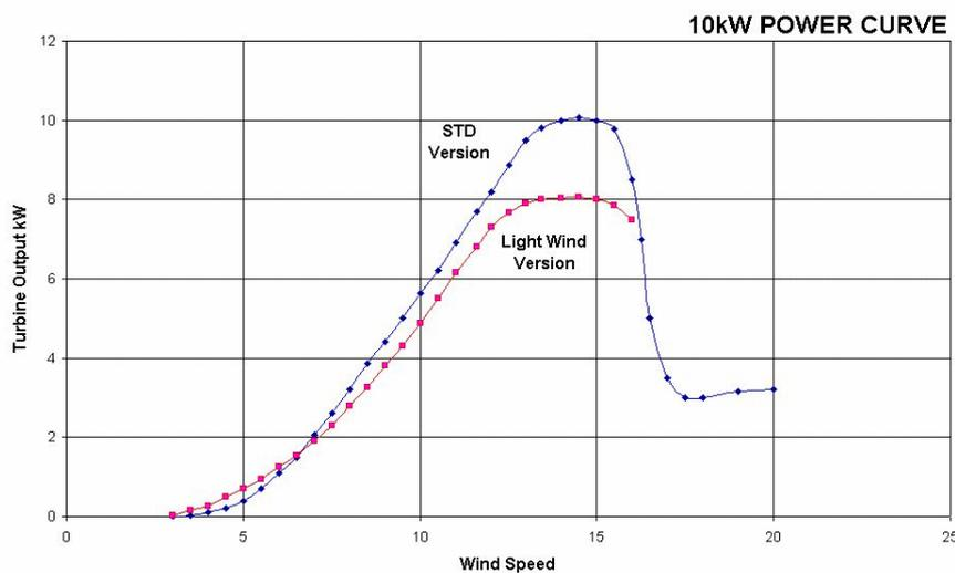
Figure 31 Wind Power and Turbine output (10 kW power curve)
