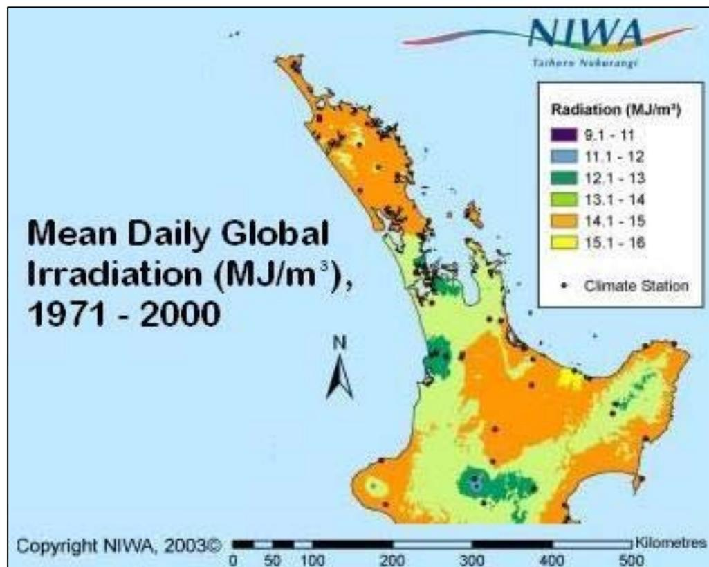
Figure 32 Mean Daily Global Irradiation ( $\text{MJ/m}^2$ ), 1971 – 2000.<sup>42</sup>
