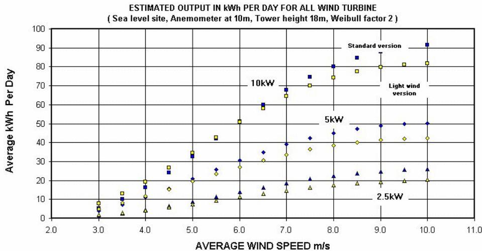
Figure 30 Estimated output in KWh per day for all wind turbines
