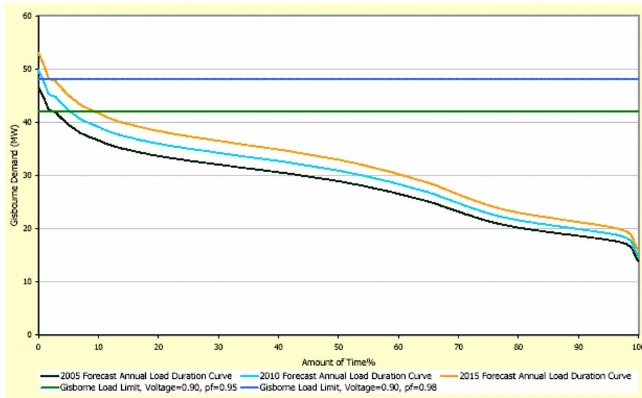
Figure 4 Gisborne Load Limits and Forecast Load Duration Curves<sup>15</sup>
