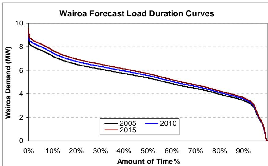
Figure 3 Wairoa Forecast Load Duration Curve<sup>14</sup>
