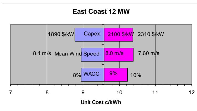
Figure 29 East Coast (typical site) 12MW
